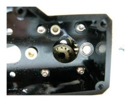
Step 7. Now find the main output shaft. Install the large gear onto the shaft like shown below. Insert the small brass spacer onto the shaft in front of the large gear. Install the other smaller brass spacer onto the shaft as well. Then install the washer that came off the gear you removed from the R2.
