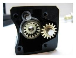
**Step 6.** Carefully assemble the 2 speed unit to the main transmission case. Reuse the 4 screws you removed earlier to reinstall the 2 speed. Make sure that you align the double gear shaft into the bearing in the main case. If the gear in the 2 speed falls down inside the case, use a screwdriver to slide it back into place.
