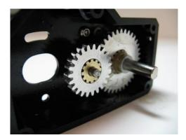
Step 11. Reinstall the front cover of the R2 2 speed. Use the screws you removed in step 1 to secure the cover. Make sure the pin lines up and the output shaft fits correct.
