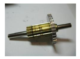
**Step 8.** Install the gear into the main case and then into the 2 speed unit. See the photos below.
