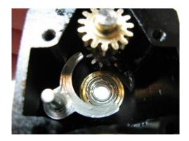
Step 5. Now you can insert the spring onto the dig collar. Install the gear you assembled in step 3 onto the dig collar. Make sure the female teeth are facing forward. There is a small groove in the gear that fits into the collar. Make sure when done that it looks like the second photo.
