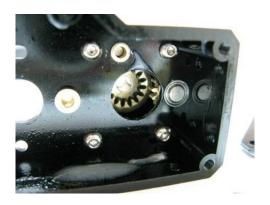
**Step 3.** Below you can see the parts you need to rebuild the 2 speed case. The spring is a part that you will need to reuse. Assemble the two gears together like shown in the second photo. To help keep everything together use a small amount of Monster lube.
