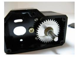
Step 9. You can now install the gear pin into the case. Now slide the new bushing onto the pin.
