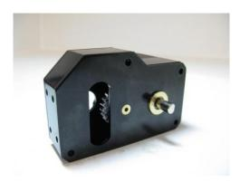
Once the cover is installed, turn the output shaft and make sure everything is spinning inside the case. Try and shift the 2 speed and make sure everything is working correct here as well. If you have any issues with either of these, remove the screws and look for any issues, and follow the directions again.
