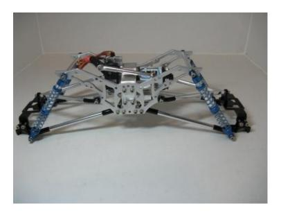
Step 11. Installation of the axles
