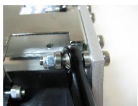
Tip. If the links are to close to the skid plate, you may have to bend the plate a small amount.
