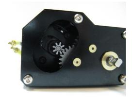
Proper gear mesh can make the R2D gears last a long time, and will reduce gear noise. If you set the lash to tight it will wear the gears and be very loud. The mesh in the photo is just about right. You will want to use some Monster Lube to lubricate the gears. More lube is better.
