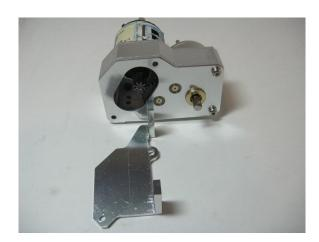
Remove the two screws on the R2D that are above and below the front hole. With these screws removed you can install the servo mount like shown in this photo. Reinstall the screws to secure the servo mount. \*
