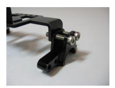
Now you can remove the old 4 link mount and install the new Single point 3 link mount. Remove the screws holding the 4 link in. Install the 3 link in the same location with the same screws. \*
