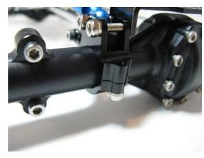
Step 12. Servo and Servo Mount Install
