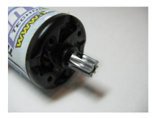
Next install the motor into the tranny on the side with the small hole. Using the black motor screws supplied insert the screws thru the holes in the tranny then into the motor. Make sure to tighten the screws only part way. You will want to align the pinion and R2 gear mesh, then tighten the screws all the way down.
